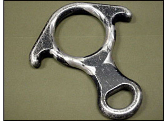
Damaged Figure 8 plate
