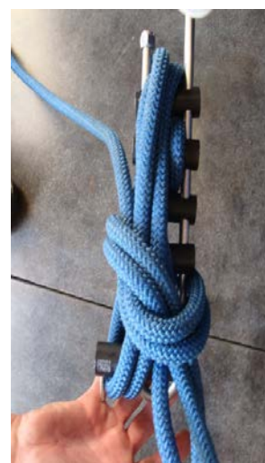
Brake Bar Rack properly tied-off
