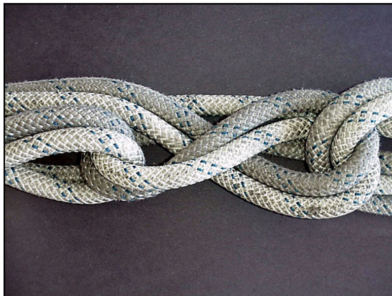
Moderate wear. Note the oil spots
