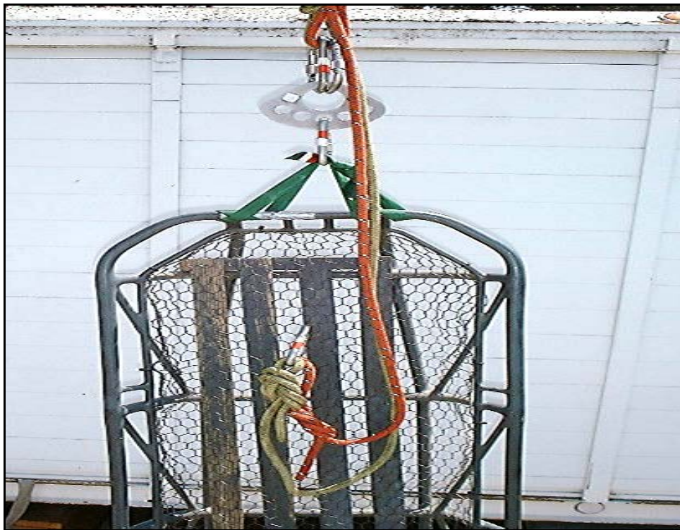
Vertical Stokes rigging without Attendant
