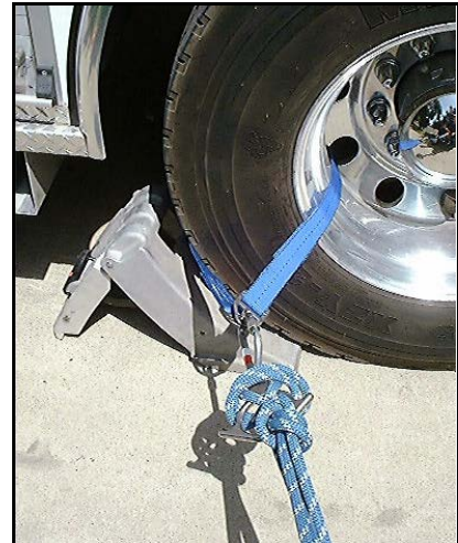
Apparatus anchor. Note the wheel is chocked.
