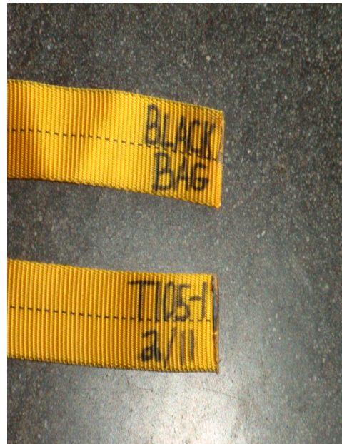
Webbing ends marked with service date and Engine assigned
