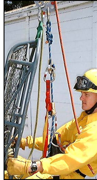
Tender Line as Main Attachment
