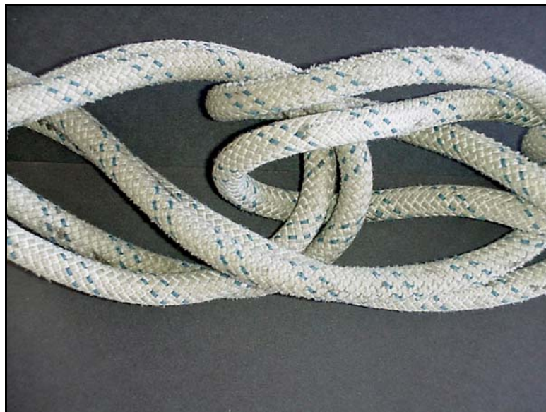
Note soft spots and oil marks in the upper right portion of the frame.
