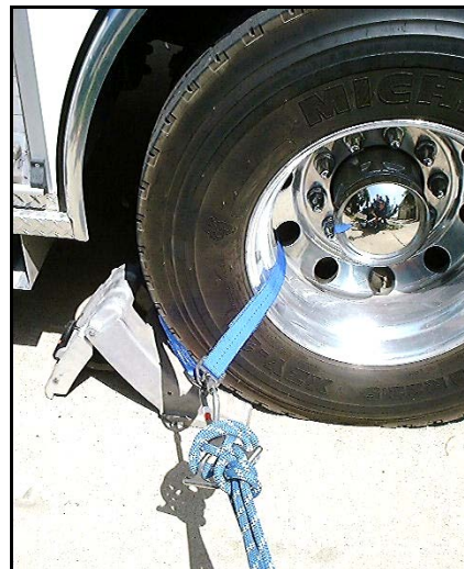
Single person load (option). Note the wheel chock under the tire to secure the vehicle.
