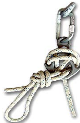
Figure 8 Descender properly tied- off
