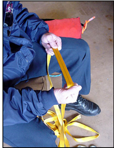
Use a similar technique to inspect webbing.
