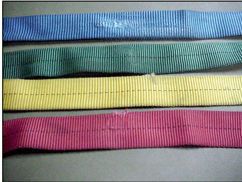
This webbing has cuts and abrasions
