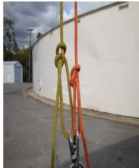
Main and Belay attached to rigging plate
