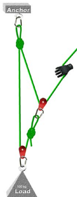
4:1 Compound System (2:1 pulling on a 2:1)
