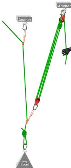
4:1 Compound Piggyback with Double pulleys
