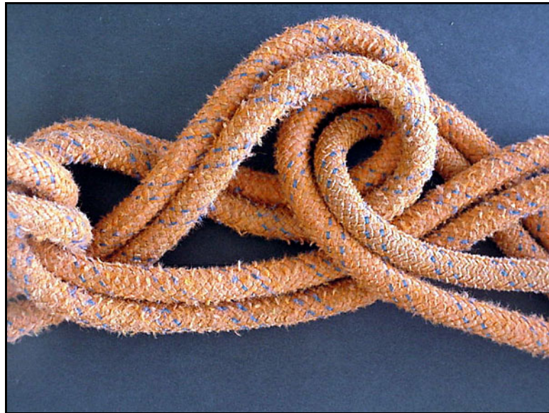
Rope with heavy wear or excessive abrasion.
